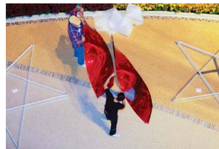
Six hundred strips of Eastman Spectar™ copolyester were heated and hand-shaped to a positive mold to give it the twister shape.
