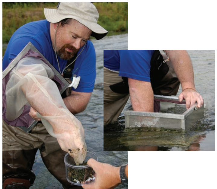
Above: Brett Marshall using a Portable Invertebrate Box Sampler (PIBS) to collect aquatic insects in shallow riffles at Zone 4. Rocks within the sampler are scraped and macroinvertebrates swept by the current into a large net attached to the PIBS.
