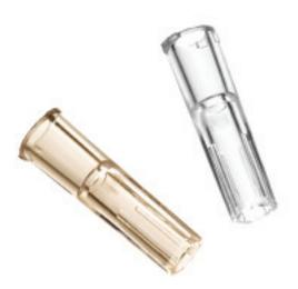
Eastman™ specialty plastics provide the best overall performance in maintaining color integrity post gamma sterilization when compared to competitive plastics, as demonstrated by the luer on the right.
