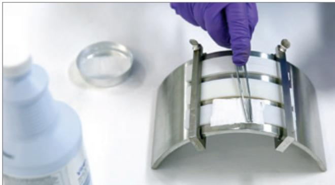
Step 3: Apply chemicals such as commonly used hospital disinfectants, lipids, drugs, or drug carrier solvents to the flex bars using a presoaked piece of cotton. Enclose the entire sample jig in a plastic bag to prevent evaporation and leave at room temperature for 24 hours.
