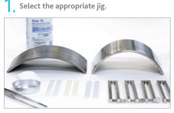
Step 1: Simply select a jig with the appropriate strain level.
