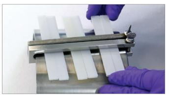
Step 2: Load plastic flex bars onto the jig. Remember to load some control samples that will not be exposed to chemicals.
