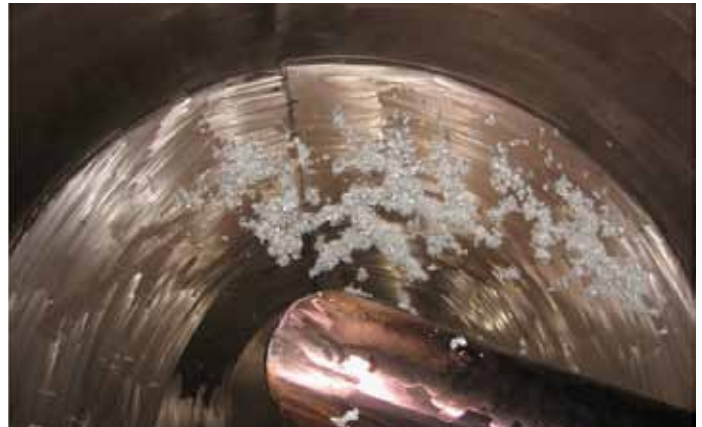
PCR flake with 1% PETG PCR flake with 1% PETG – inside of dryer cone after testing. Significant sticking is noted.
