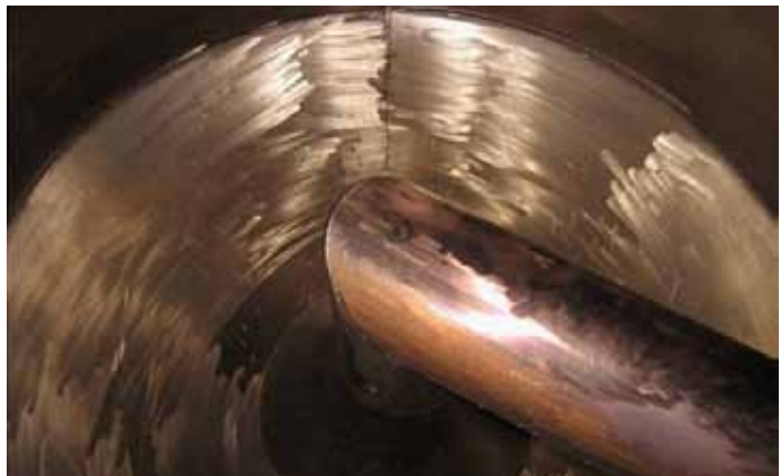
PCR flake with 25% Eastman Aspira™ copolyester EN177 – inside of dryer cone after testing. No sticking to dryer sidewalls is observed.
