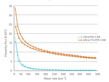
A Bohlin rheometer with a 40 mm, 1 degree cone geometry was utilized to conduct a continuous linear shear ramp from 0 to 500s-1 over 60s then back to 0s-1 over a further 60s in a controlled rate mode. A temperature of 25°C with a 60s pre-shear delay at 0s-1 was employed and 30 sample points per minute were recorded giving a total of 60 measurements.
