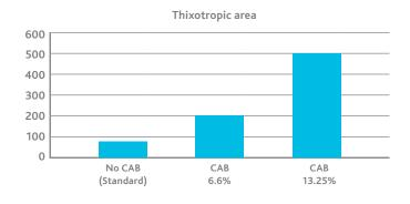
Eastman<sup>™</sup> CAB cellulose ester increases the thixotropic area. As stated previously, this should produce anaerobic adhesives with increased flow after shearing.
