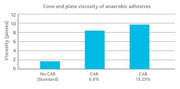
Adding Eastman<sup>™</sup> CAB 551-0.2 cellulose ester increases the very high shear cone and plate viscosity. This may enable a formulator the option of producing an adhesive that has greater resistance to spreading after the tightening operations involved with threaded pipes, nuts and bolts.
