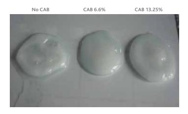
The formulation with fumed silica alone produced separation of liquid component after storage at ambient conditions. This is clearly demonstrated on the glass panel above.
