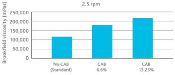
Brookfield measurements at 23°C (spindles #3 to #6 @ 2.5 rpm-30 rpm)
