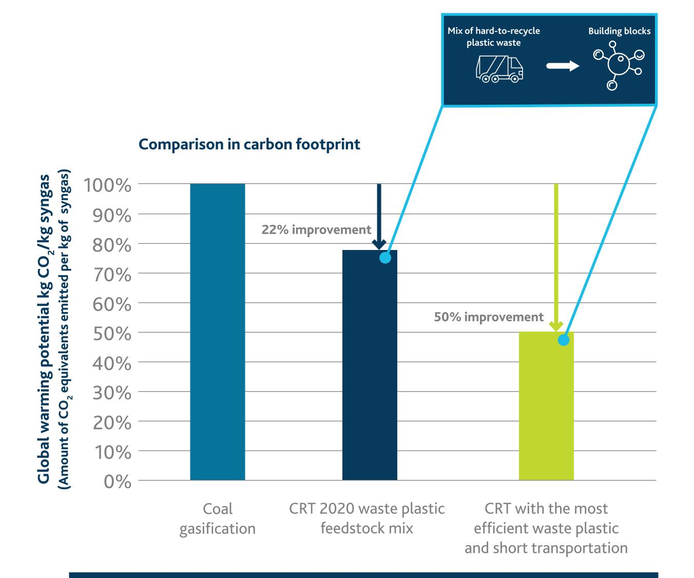
By using waste plastic as a raw material to replace conventional fossil-based feedstocks, CRT can reduce the GHG emissions for syngas production to 20%–50%.
