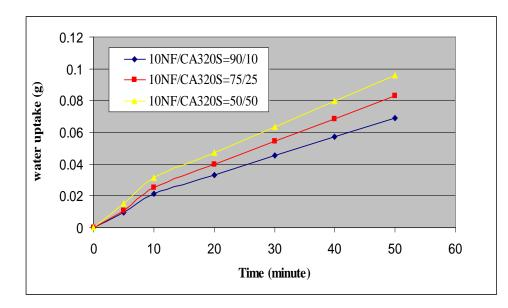
Figure 1. The ratio of CA-398-10 NF/EP to CA-320S NF/EP effect on the permeability of the coating films (PEG400 = 11.1% in the formulations).
