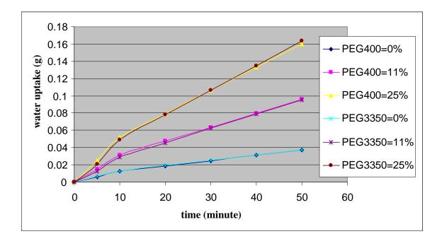
Figure 2. PEG level and molecular weight effect on the permeability of the coating films. CA-398-10 NF/EP/ CA-320S NF/EP = 50/50; acetyl in 10 NF/EP = 39.4%.
