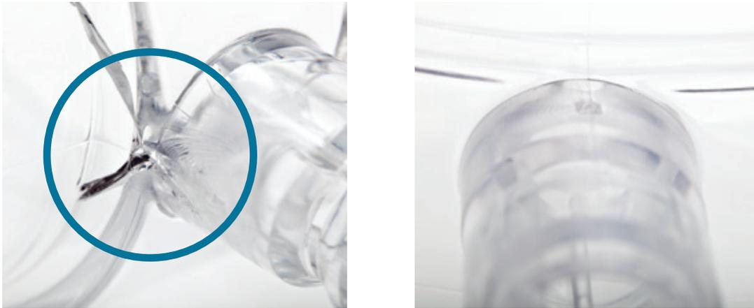
*The PC housing on the left shows a significant crack (visible in circled area) after eight hours of exposure, indicating chemical attack due to high residual and molded-in stress in the part. The housing on the right, molded with Tritan, has not cracked after 120 hours of exposure.*
