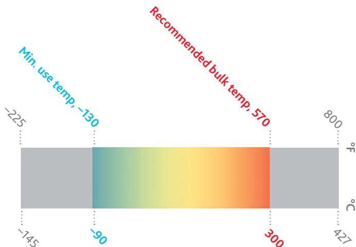
Covering a temperature range from  $-90$  to  $300^{\circ}\text{C}$  in a heat transfer circuit with a single heat transfer medium poses a real challenge. To solve this, physical parameters of the medium should be optimally coordinated. Eastman Marlotherm® XC heat transfer fluid meets these conditions in an optimum way.
