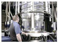
With EVO Ultra Die technology, Reifenhäuser Blown Film sets a new standard for the fastest barrier blown film die head in the market. Its new die head concept now allows the production of even more layers.
