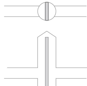
Make drop larger than supply feeder so that area of half the drop does not restrict feeder. Do not oversize to point of reducing velocity where laminar flow can result.
