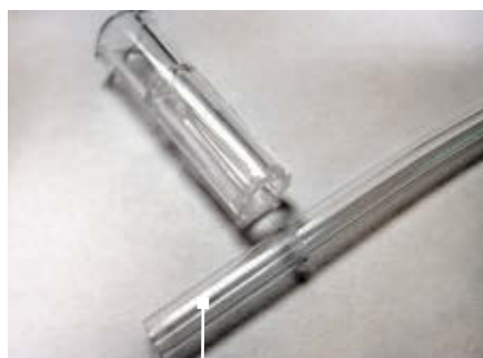
Tubing delaminates from luer.
