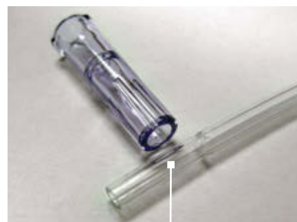
Tubing delaminates from luer.
