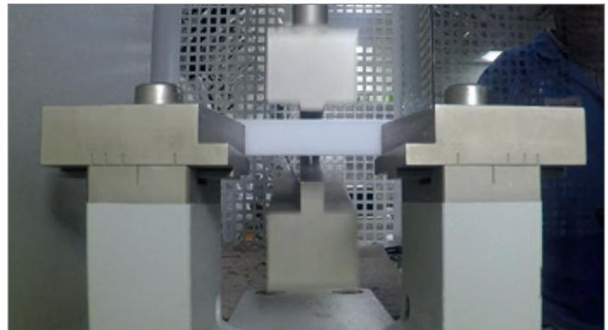
Step 4: Unload the samples, and run a reverse side impact test on the exposed and control samples.
