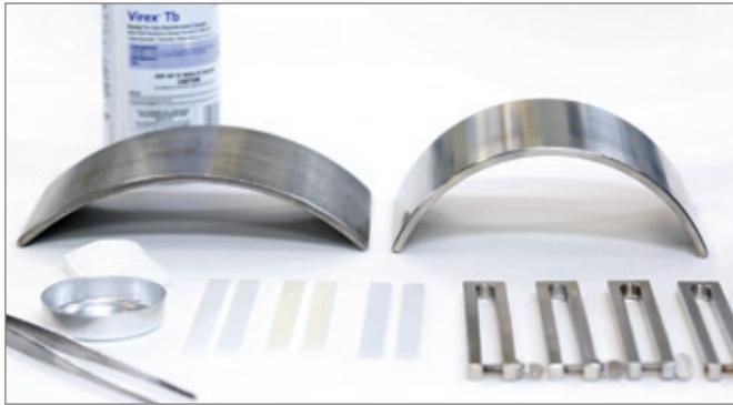
Step 1: Simply select a jig with the appropriate strain level.
