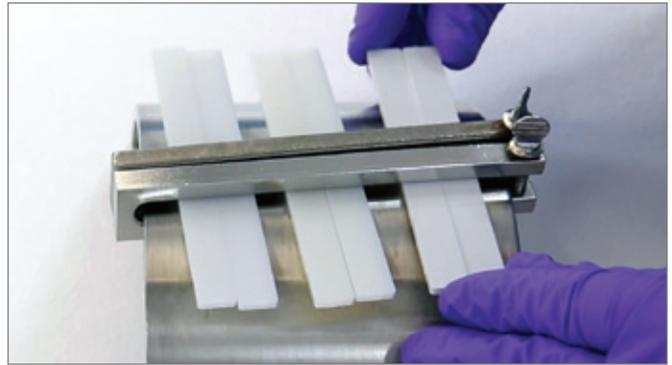
Step 2: Load plastic flex bars onto the jig. Remember to load some control samples that will not be exposed to chemicals.
