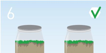
6 Inspect the jars for germination in 1 to 3 days. The soil is safe for planting if seeds in the treated jar germinate normally compared to the untreated check.
