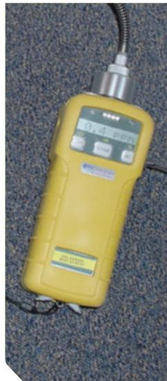
response factor/correction factor. The lower this factor value the more sensitive the P.I.D. for the measured compound.
