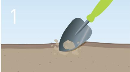
1 With a trowel, dig into the treated soil to, or just below, the depth of application.
