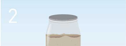
2 Remove 2 to 4 small (25 - 50 g) treated soil samples, mix lightly, and immediately place a portion in an airtight jar so that fumes will not escape. Use glass jars with gas-tight lids.
