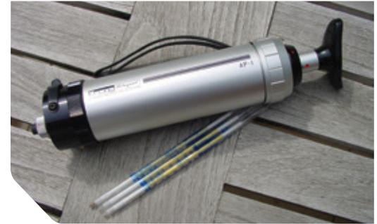
Depending on manufacturers' instructions a volume of ambient air is pumped through a sealed glass gas reaction tube after inlet and exhaust (pump-side) tips are broken off. The gas reacts with a colouring agent sorbed on carrier material. Readings are made of the discoloured zone on a numeric MITC concentration scale.
