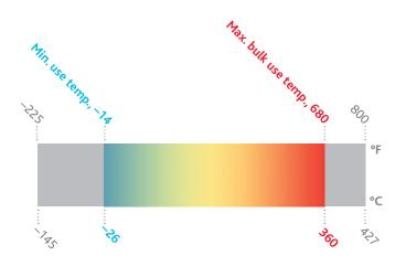
Eastman Therminol<sup>®</sup> 68 heat transfer fluid is a high-temperature fluid with excellent thermal stability. Therminol 68 was developed for use at temperatures up to 360°C (680°F) in liquid phase heat transfer systems. Static pressure of about 2 bar should maintain the liquid phase at high temperatures.
