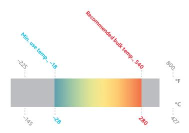
Eastman Therminol® 54 heat transfer fluid is a synthetic fluid designed to provide reliable, consistent heat transfer performance over a long service life at a recommended bulk temperature of 280°C (540°F).
