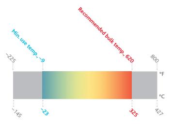
Eastman Therminol<sup>®</sup> 62 heat transfer fluid offers outstanding performance to 325°C (620°F), including excellent thermal stability and low vapor pressure. These properties result in reliable, consistent performance of heat transfer systems over long periods of time. The performance of Therminol heat transfer fluids has been proven through many years of industrial experience under a wide range of operating conditions.
