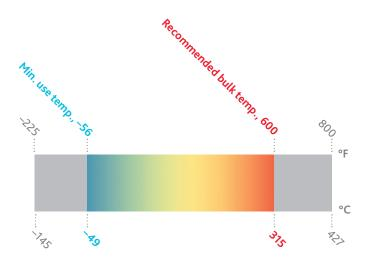
Eastman Therminol<sup>®</sup> 59 heat transfer fluid offers excellent low-temperature pumping characteristics (pumpable at –49°C/–56°F) for problem-free start-ups in cold climates while offering thermal stability at a recommended bulk temperature of 315°C (600°F).
