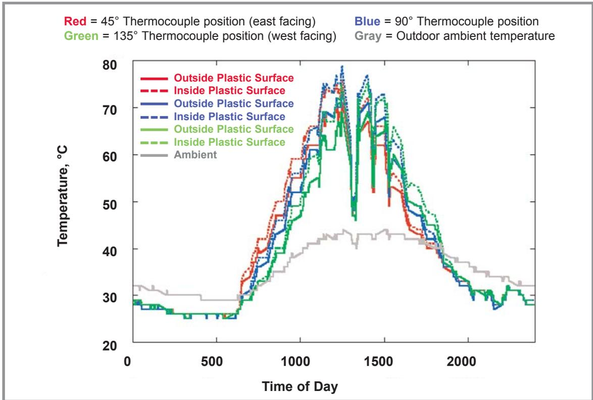
Figure 7: Clear-Clear Double Dome Temperature Curve
