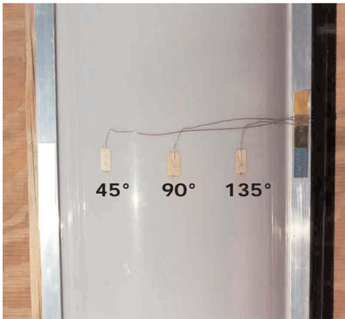
Thermocouples were attached to each dome (inner and outer surfaces) at 45°, 90°, and 135° with respect to ground level (see Figure 1). The positions were varied to account for the curved shape of the domes and the position of the sun at different times of the day. The 45° position thermocouple was placed in an Eastern facing direction, the 135° in a Western direction. The skylights were positioned flatwise on a solid wooden platform (Figure 2).
