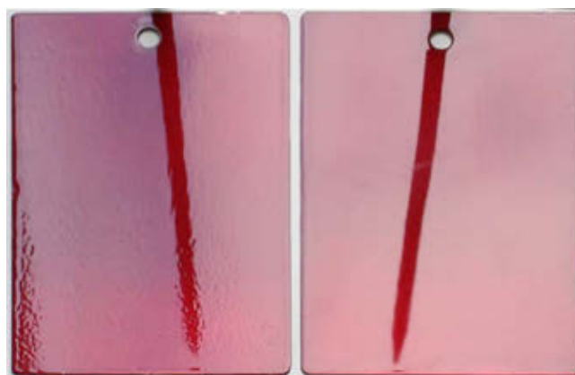
Panel without Eastman CAB-551-0.2—orange peel/less reflection
