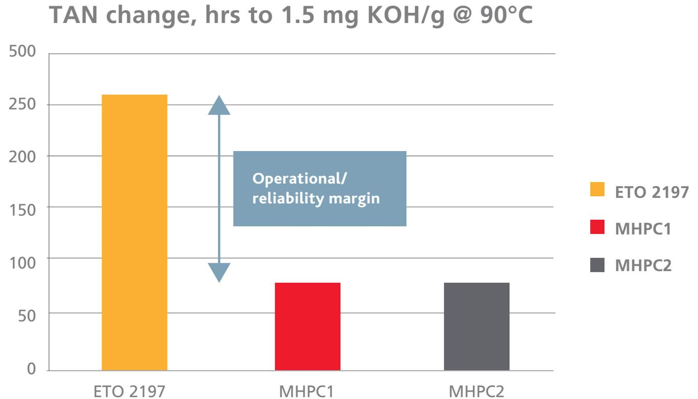
*TAN change is an excellent measure of an oil starting to rapidly degrade. Test results from the Cyclic Coker Mister—consistent with industry tests such as GE Alcor.*
