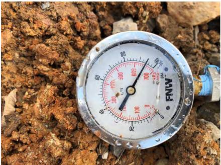
(2) IW influent piping (2" HDPE) to CTS#3 was pressure tested prior to system startup. Test pressures were maintained for the duration of the 60-minute tests. No leaks were detected during pressure testing.
