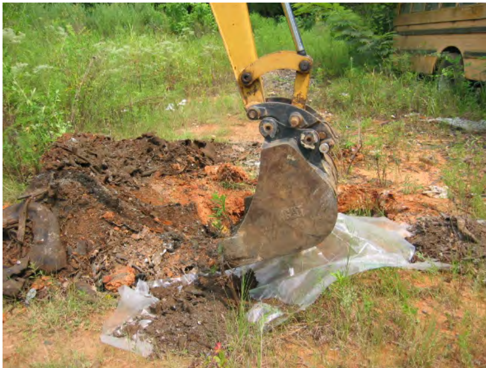
Photograph 4 – Auto fluff debris excavated from test pit is shown adjacent to the pit and within the bucket of the backhoe.
