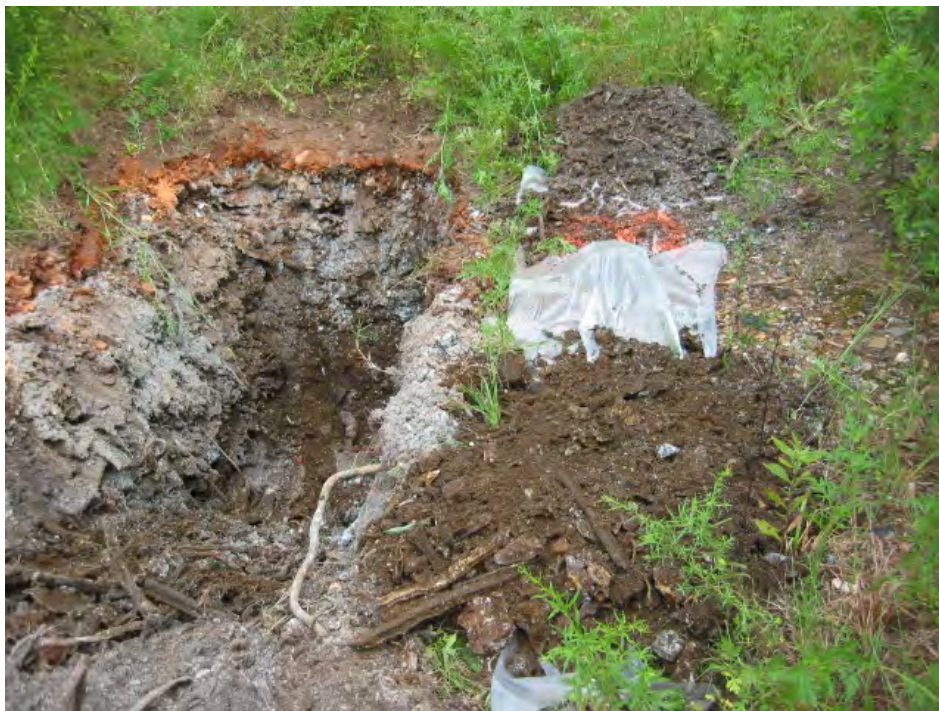
Photograph 3 – Test pit excavation showing discolored auto fluff debris.
