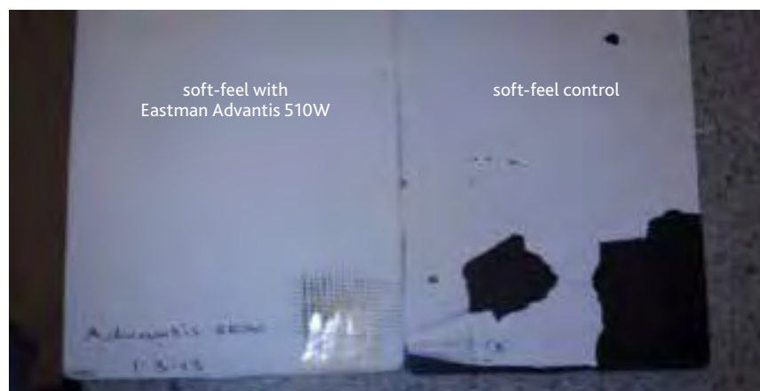
Figure 1: Side by side comparison of the coated substrates
