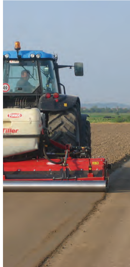
Soil compacting rolls on IMANTS machines (left) and on a FORIGO machine (right)
