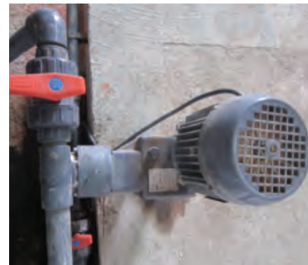
Alternatively, a pump can be connected directly to the drum containing metam (most common method).
