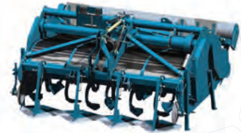
Rotary spading machine with injection (manufactured by Imants)
