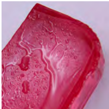
Figure 1. A section of hot-melt strippable material that is leaching oil
