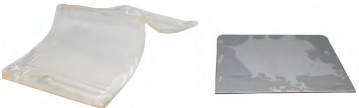
Figure 5. Peeled-off hot-melt strippable coating (formulation 2) shows no damage to the metal. An oil film is visible.
