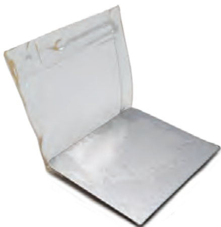
Figure 4. The edges of the coatings (formulation 2) are cut, allowing the coating to be peeled off.
