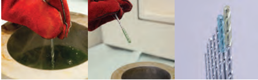
Figure 2. End of a metal drill bit dipped in the hot melt, cooled and handled
