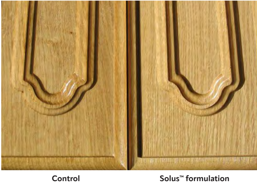
Figure 4. Properties of the coating systems on oak panels
