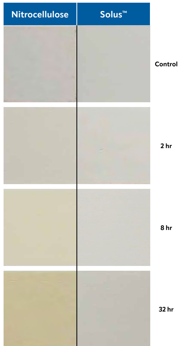
Figure 1. UV stability of white wood lacquer based on Eastman Solus™ vs. nitrocellulose
