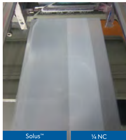
Figure 4. Comparison of clogging of Solus™-based and NC-based inks
