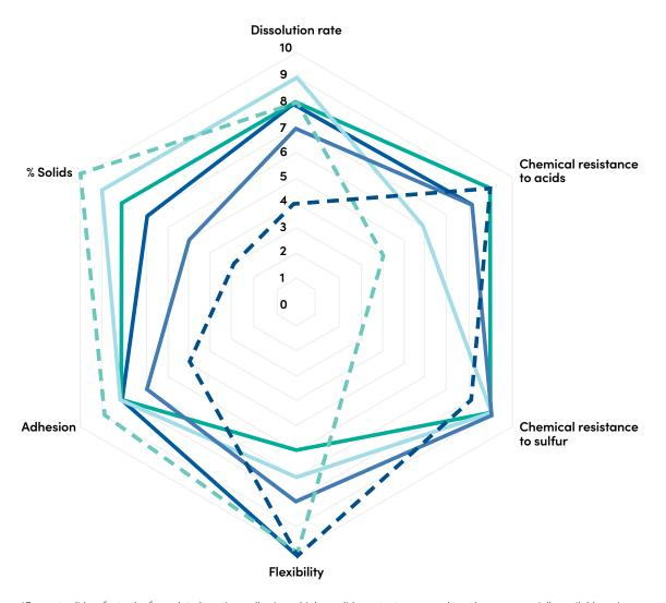
High T<sub>a</sub>, high molecular weight 49% solids\* Low T<sub>a</sub>, medium molecular weight 62% solids\* Tetrashield MP2100 58% solids\* **Tetrashield MP2101** 51% solids\* **Tetrashield MP2303** 57% solids\* **Tetrashield MP2104** 54% solids\*
