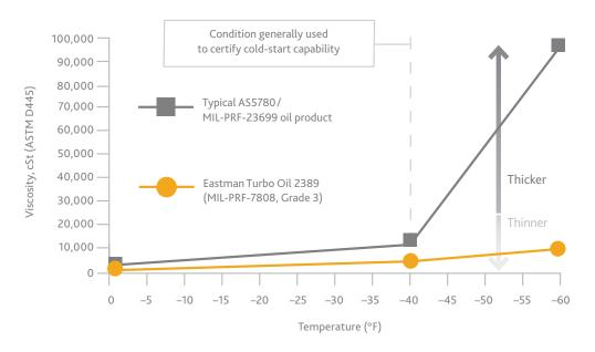
Many large commercial airlines use ETO 2389 in their auxiliary power units (APUs) because of the reliability it affords this equipment when starting after long, cold soaks at altitude. By using ETO 2389, your airline can meet the requirements from regulatory agencies for ETOPS operations.
