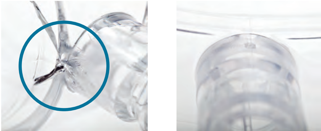
Figure 1. Medical device housing after exposure to Virex TB
