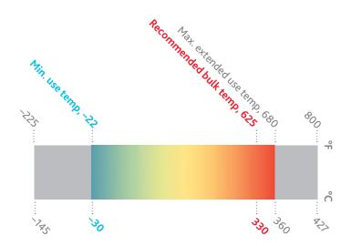
Eastman Marlotherm® LH heat transfer fluid is a low-viscosity, synthetic organic heat transfer medium for use in both the liquid and vapor phase for closed, forced-circulation heat transfer systems.
