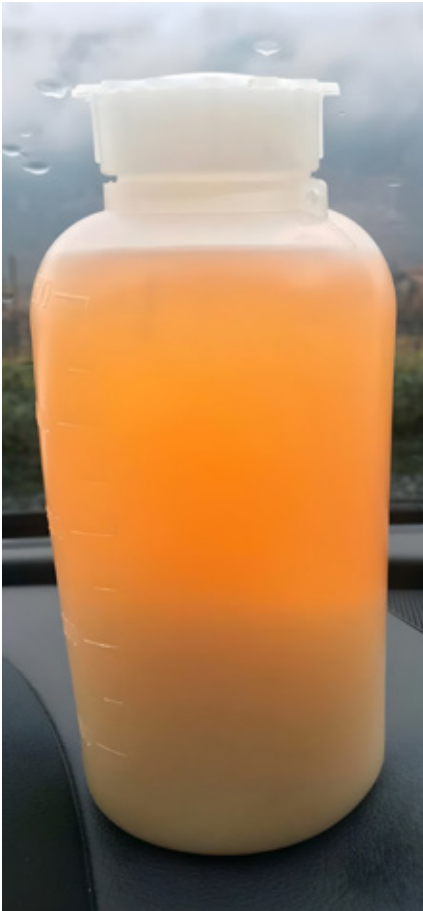
Sample of new material showing solid/liquid-phase separation and formation of waxy solids.
