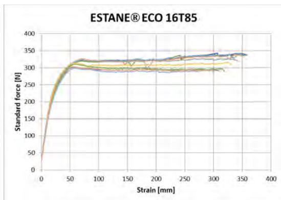
**Figure 3.** Adhesion strength traces of ESTANE<sup>®</sup> ECO 16T85 overmolded onto Tritan™ TX1501HF. The average adhesion strength value calculated from this data was found to be 311 N.
