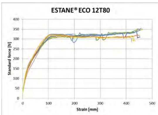
**Figure 4.** Adhesion strength traces of ESTANE<sup>®</sup> ECO 12T80 overmolded onto Tritan™ TX1501HF. The average adhesion strength value calculated from this data was found to be 316 N.
