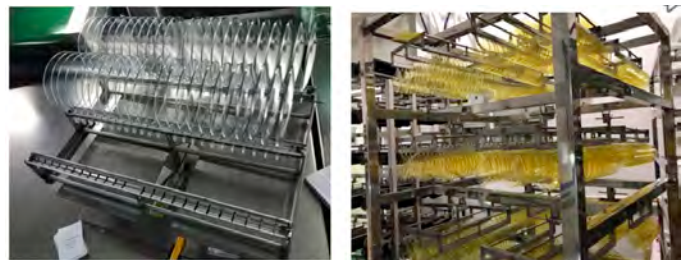
Figure 8. Lens transport in manufacturing plant
