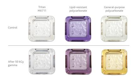
Tritan shows minimal color shift and returns to original color in 14 days. Acrylic and PC have significant color shifts after exposure to gamma radiation.
