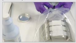
Chemicals such as commonly used hospital disinfectants, lipids, drugs, or drug carrier solvents can be used. Enclose the entire sample jig in a plastic bag to prevent evaporation and leave at room temperature for 24 hours.
