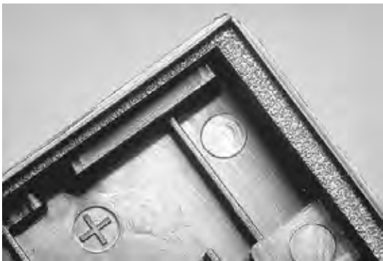
Close-up of a typical textured surface joint
