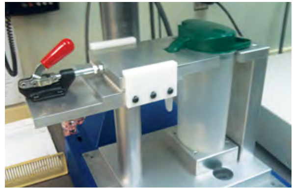
Figure 3. Examples of stabilization devices for firmly securing parts during the welding process
