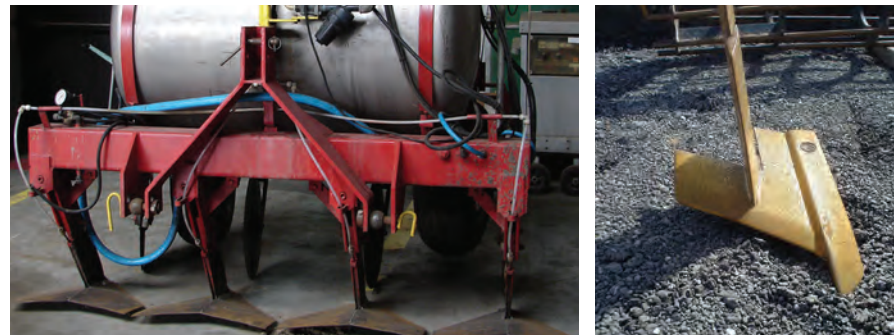
Various types of goosefoot blade injection systems
