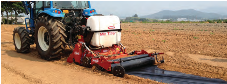
Single-pass equipment: Application/incorporation/plastic film sealing machine
