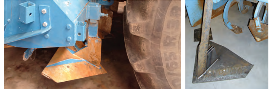
Various types of goosefoot blade injection systems
