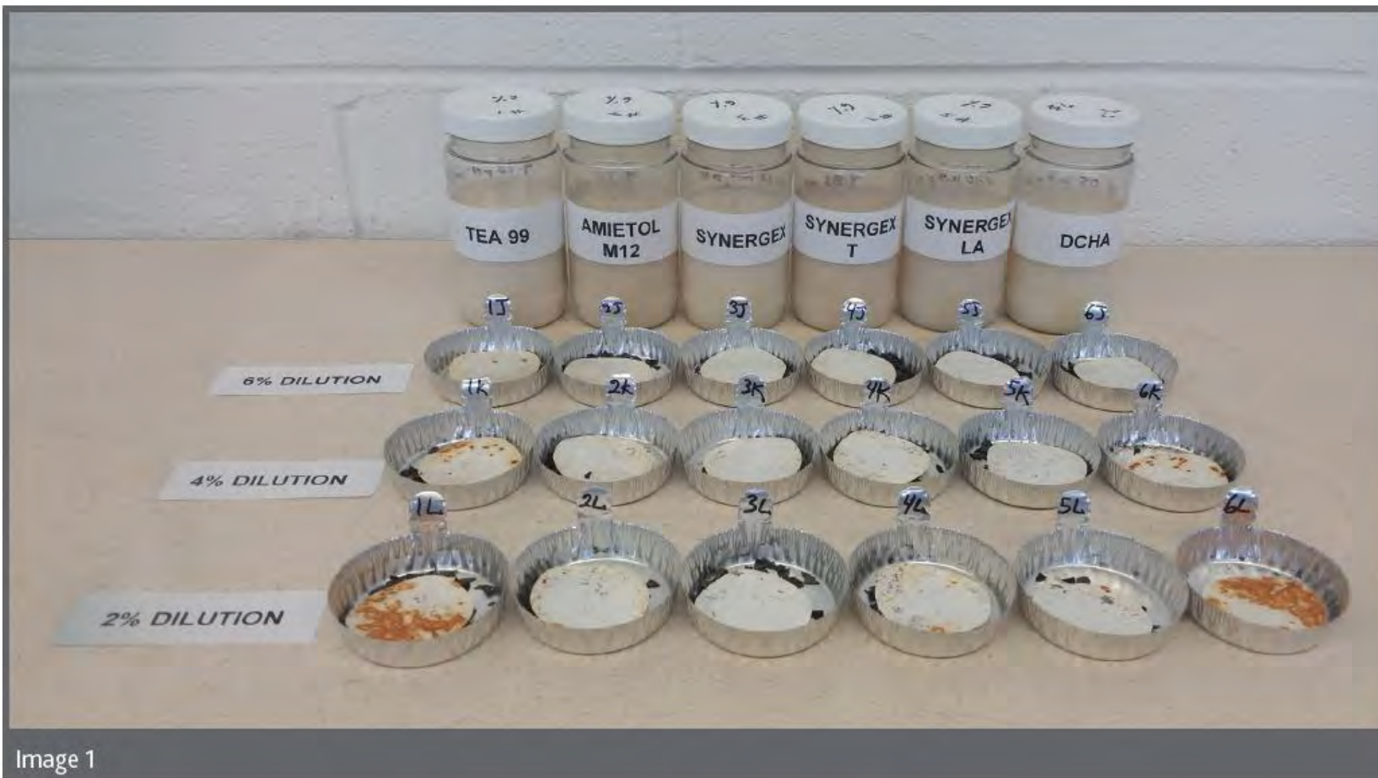
Image 1 shows results of cast iron chip tests on fluids halfway through testing (4th challenge). Fluids across the top row are at 6% concentration. Fluids in the middle row are at 4%. Fluids across the bottom row are at 2%. This is where most of the rust appears on those fluids with triethanolamine 99 and DCHA.
