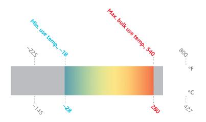
Eastman Therminol® 54 heat transfer fluid is a synthetic fluid designed to provide reliable, consistent heat transfer performance over a long service life at maximum bulk temperatures up to 280°C (540°F).
