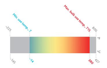
Eastman Therminol® 72 heat transfer fluid offers outstanding high-temperature performance up to 380°C (715°F) with excellent thermal stability in systems at medium pressures. Static pressure of about 6 bar should maintain the liquid phase at high temperatures. When operating in a well-maintained and operated heat transfer system, Therminol 72 can provide reliable, consistent performance over long periods of time.
