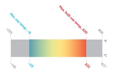
Eastman Therminol® 62 heat transfer fluid offers outstanding performance to 325°C (620°F), including excellent thermal stability and low vapor pressure. These properties result in reliable, consistent performance of heat transfer systems over long periods of time. The performance of Therminol heat transfer fluids has been proven through many years of industrial experience under a wide range of operating conditions.
