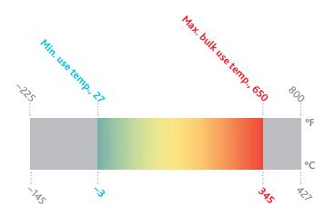
Eastman Therminol® 66 heat transfer fluid offers outstanding high-temperature performance to 345°C (650°F), including excellent thermal stability and low vapor pressure. These properties result in reliable, consistent performance of heat transfer systems over long periods of time. Therminol 66 performance is proven through many years of industrial experience under a wide range of operating conditions. No heat transfer fluid material in the world has had more success than Therminol 66.
