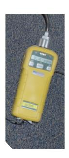
response factor/correction factor. The lower this factor value the more sensitive the P.I.D. for the measured compound.
