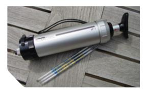
Depending on manufacturers' instructions a volume of ambient air is pumped through a sealed glass gas reaction tube after inlet and exhaust (pump-side) tips are broken off. The gas reacts with a colouring agent sorbed on carrier material. Readings are made of the discoloured zone on a numeric MITC concentration scale.
