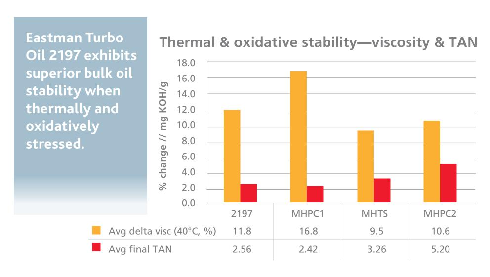
Improved oxidative stability leads to longer oil life and improved operations for an engine.
